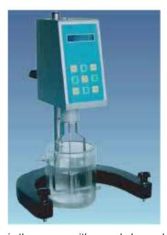
Direct Readout of all measurement parameters on an illuminated Liquid Crystal Display • Data on screen: • Speed selected: r.p.m. • Spindle selected: S.P. • Viscosity reading: cP (mPa-s) • Percentage of full scale: SR -Shera stress (with special spindles): SS -Determination of relative viscosity and absolute viscosity compute yield stress • Different menu options • AUTO TEST of the equipment by scanning at different speeds, with audible and visual warning if it is not operating properly
