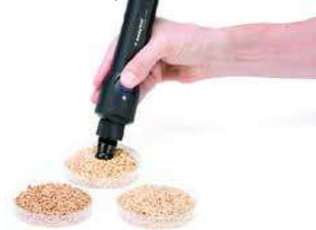
Portable Nano NIR in application
