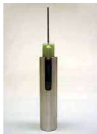
Fig.4 Measure the falling time between two markings on the extension bar attached to the needle.
