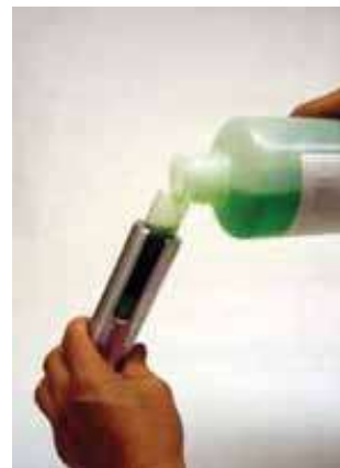
Fig.2 Pour the sample into the syringe up to the top of the viscometer main body.
