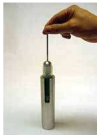
Fig.3 Insert the needle into the syringe until the top of the needle reaches the top of the syringe and then drop the needle.
