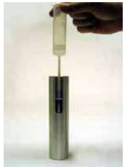
Fig.1 Slide the syringe into the viscometer main body.
