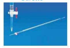
This Burette has a transparent acrylic body and a leak proof stopcock fitted with a self lubricating PTEE plug. Each Burette is individually calibrated to give maximum accuracy. Acrylic body is unaffected by dilute minerals acids & bases except Hydrofloric Acid & Ammonium Hydroxide. The pH range of 1-14 is deal and can be used upto 5% wt/wt of acids or 30% bases.
