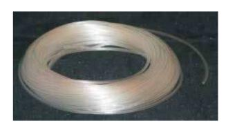
Crystal clear and flexible. Tygon laboratory tubing handles virtually all inorganic chemicals found in the lab. It is non-oxidizing and non-contamination. This tube can be autoclaved and is flexible even at-43°C. Durometer hardness shore A55. Can be used with condensers, incubators, gas lines, drain lines etc.
