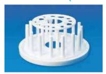
This rack is an excellent lab apparatus compatible with different sizes of tubes. Four sides of this rack can be used for tubes of ¢30mm, ¢20mm, ¢17mm & ¢12mm
