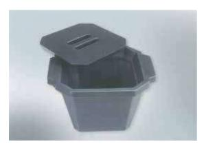
Durable rigid ice bucket is unbreakable in normal use. Excellent insulating properties. Suitable for use with liquid nitrogen, dry ice, water-ice salt solution and acetone.
