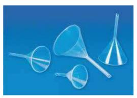
Autoclavable Funnels designed for use with standard filter paper. The funnel body is at  $60^{\circ}$  angle with internal ribs at  $58^{\circ}$  for rapid filtration. External ribs prevent air locks
