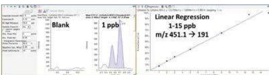
Figure 6: Integration parameters in MultiQuant 3.0.2 for Cyfluthrin acquired on a + system with a 25µL injection showing multiple isomers.
