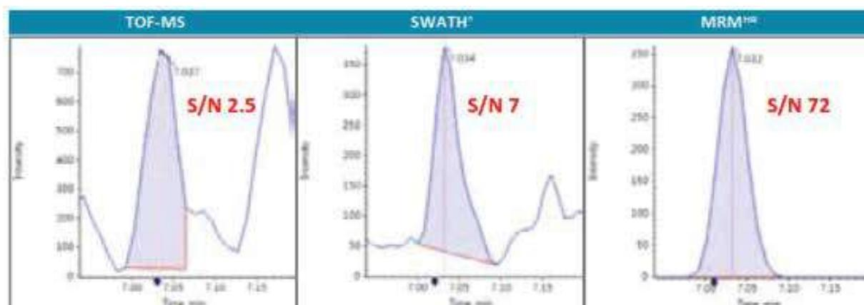
Figure 4: Extracted ion chromatograms of azithromycin spiked at 0.2 ng/mL in liver extract from different acquisition experiments. Left panel: TOF-MS ( $m/z$  749.5158). Middle panel: SWATH -MS/MS (749.52 > 591.4215). Right panel: MRMHR (749.52>591.4215).
