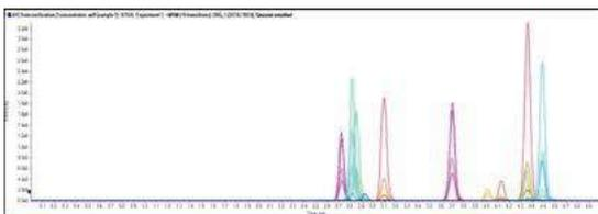
Figure 8B: Elution profile of target cannabinoid analytes in solvent using the same mobile phases and analytical column as the pesticide panel
