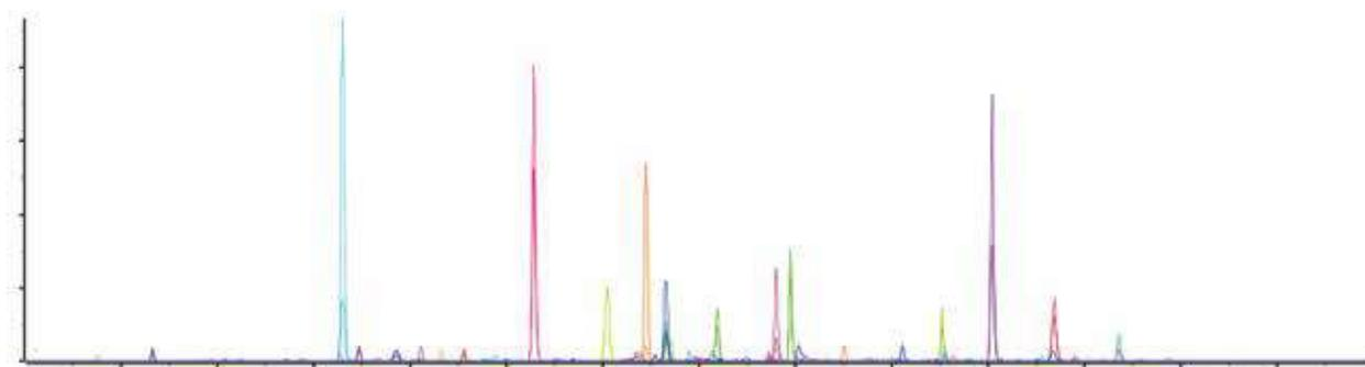
Figure 2. Extracted ion chromatograms from the LC-MS/MS analysis of raw meat mixture containing pork, beef, lamb, chicken, duck and horse (10, 20, 20, 20, 20 and 10% w/w, respectively). Multiple peaks corresponding to tryptic marker peptides are displayed.
