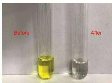
Figure 3. Sample preparation and clean up. Visual comparison of a grain sample before and after the Cleanert SPE column clean-up step. Cleaning up the sample can provide reduction of matrix interferences as well as help in maintaining instrument performance.
