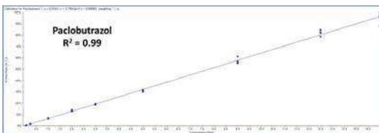
Figure 12: 5 calibration curve replicates for Paclobutrazol from 0.75-15 ppb on a + system.
