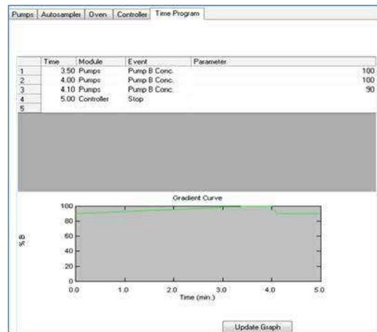
Figure 3B: LC Gradient is detailed using % Mobile Phase B as the parameter
