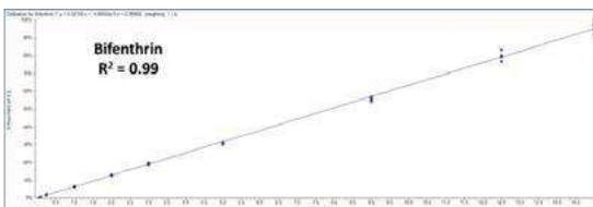
Figure 13: 5 calibration curve replicates for Bifenthrin from 0.75-15 ppb on a + system.
