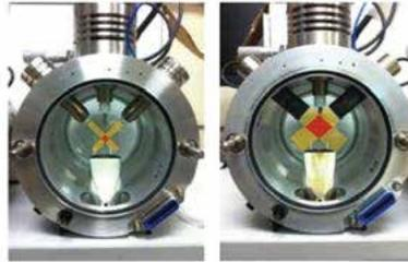
Figure 4: ATL TurboV source (left) and ATL IonDrive source (right) have different ion source temperatures that are optimal for each model.
