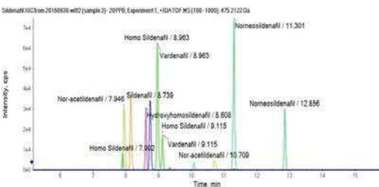
3. 8 impotence drug mixtures (20ppb), ion extraction flow diagram (XIC) appears below;
