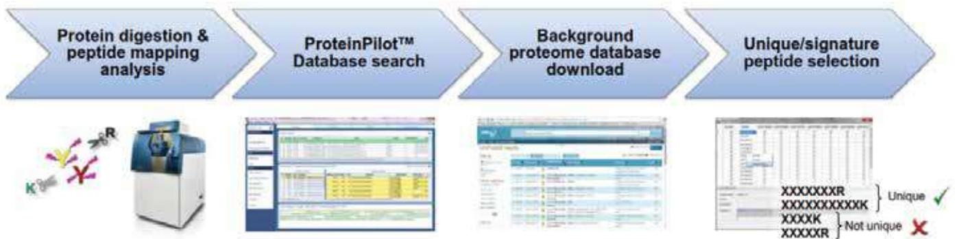
Figure 1. Signature peptide selection workflow using the ATL TripleTOF 6600 system and ProteinPilot software
