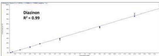
Figure 11: 5 calibration curve replicates for Diazinon from 0.75-15 ppb on a + system.
