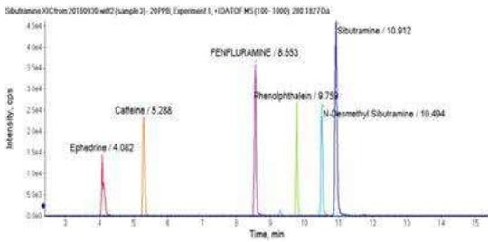
5. 5 blood pressure-lowering drug mixtures (20ppb), ion extraction flow diagram (XIC) appears below;
