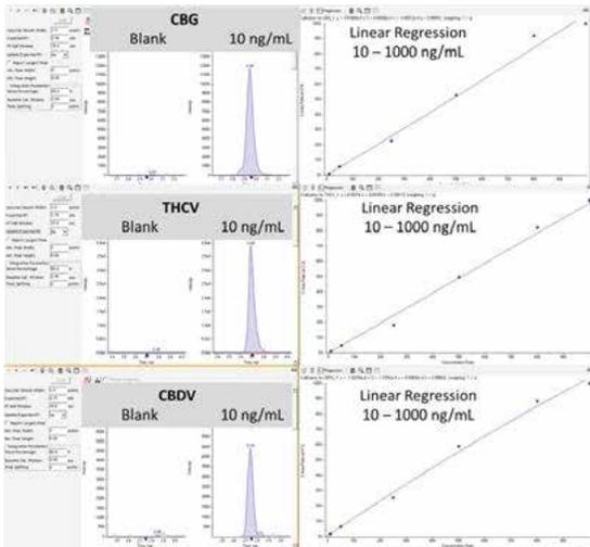
Figure 16: Representative solvent blanks, first LOQ standard and calibration linearity of CBG, THCv and CBDV.
