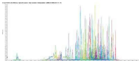
Figure 2. Chromatographic profile of MRM transitions in a standard solution of the 209-pesticide mixture in the iD quant kit. Separation was achieved using Phenomenex Kinetex XB-C18 column and a 21-minute LC gradient.
