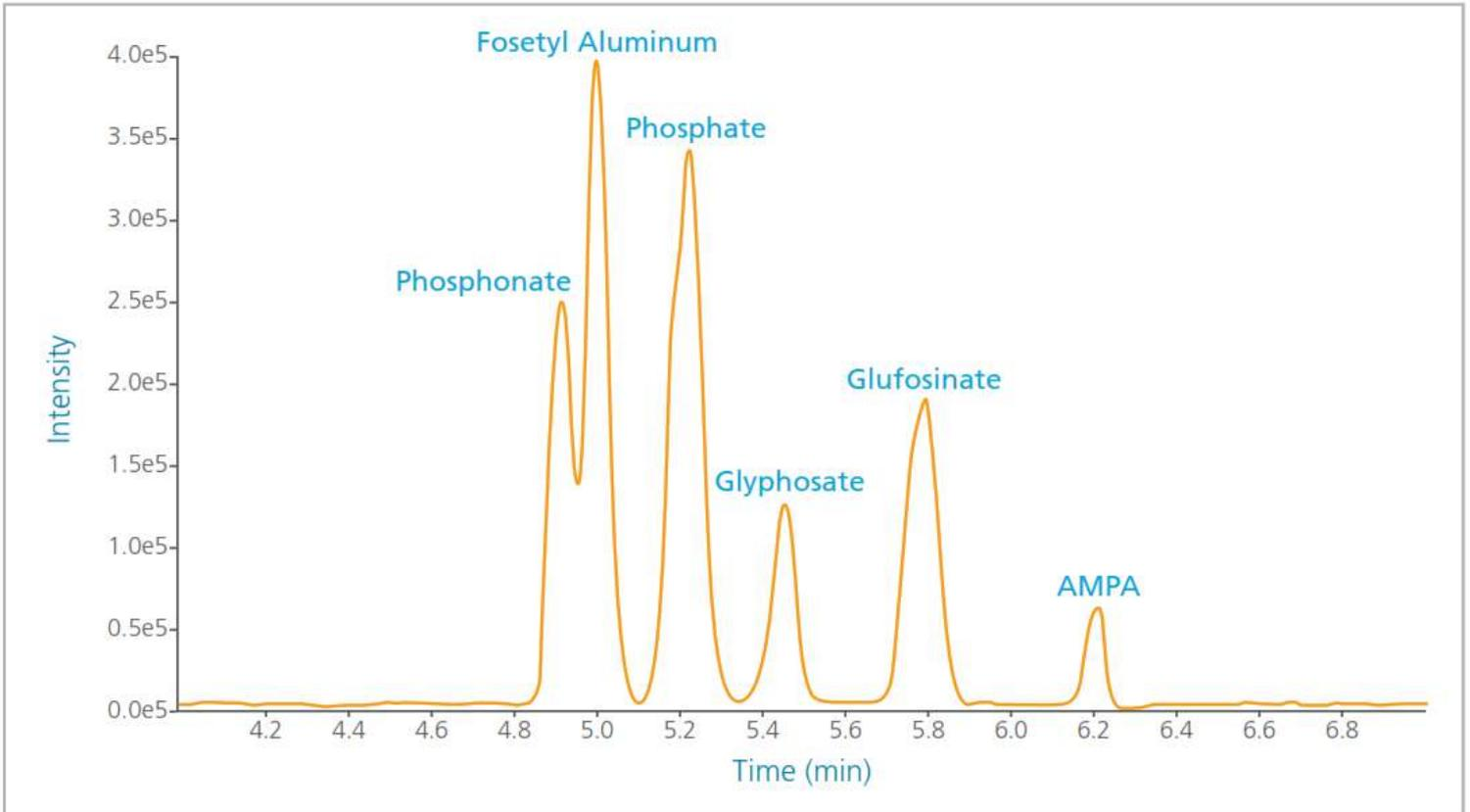
Figure 2: CESI-MS provides clear separation and detection of glyphosate and three of its degradation products: glufosinate, AMPA and phosphate, along with fosetyl aluminum and one of its degradation products, phosphonate.
