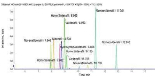
4. 6 weight loss drug mixtures (20ppb), ion extraction flow diagram (XIC) appears below;
