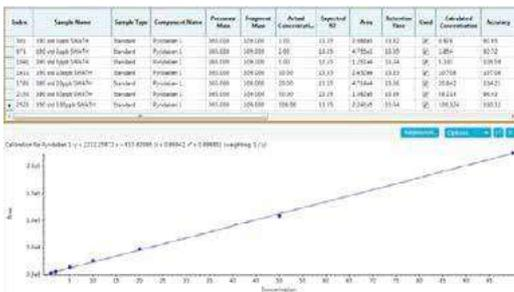
Figure 6 Quantitative linearity using pyridaben as an example
