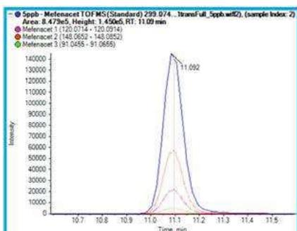
Figure 5. Ion ratios. Ion ratios for compound identity confirmation can be generated for multiple MRM transitions. In this example for Mefenacet, the TOFMS peak is overlaid with the MRM peaks extracted for three transitions, the first of which comes from the optimized acquisition channel and the last two extracted from the full- scan acquisition channel.
