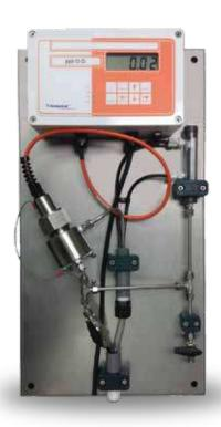
The model 3865 analyzer is designed and manufactured to give you fast response, flexibility, reliability, and ease of use. Automatic ranging reads directly in parts per billion ( $\mu g/L$ ) without any need for manual setup. The analyzer's measuring range is from 0 ppb to 20 ppm D.O.
