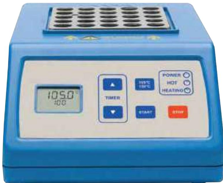
The Analytical 3980 COD reactor is constructed of durable materials. The aluminum block incorporates a 25-vial capacity and a well for a reference temperature probe.
