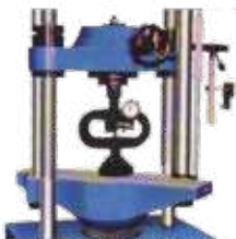
CALIBRATION OF MACHINE WITH PROVING RING
