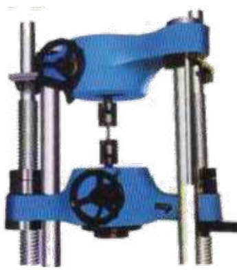
ATTACHMENT FOR TENSION TEST FOR SHOULDERED AND THREADED SPECIMENTS
