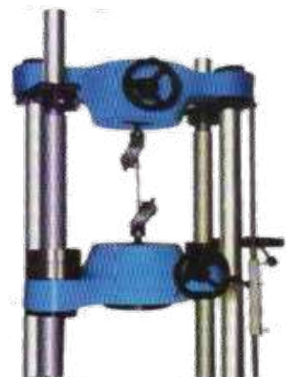
ATTACHMENT FOR TENSION TEST FOR WIRE ROPES
