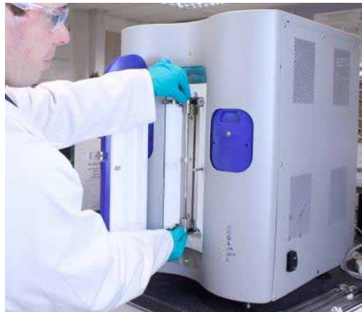
iGC-SEA straight column design - simple sample packing and column loading
