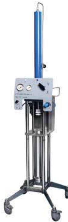
The DAC (dynamic axial compression) column adopts latest design by ATL. The piston of column always produces a stable pressure on packing bed which can effectively prevent the collapse and loose of the column bed.
