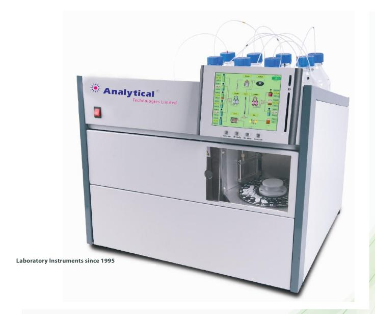
AAA 3500 is a compact device designed fodetermination of amino acids and biogenic amines.
